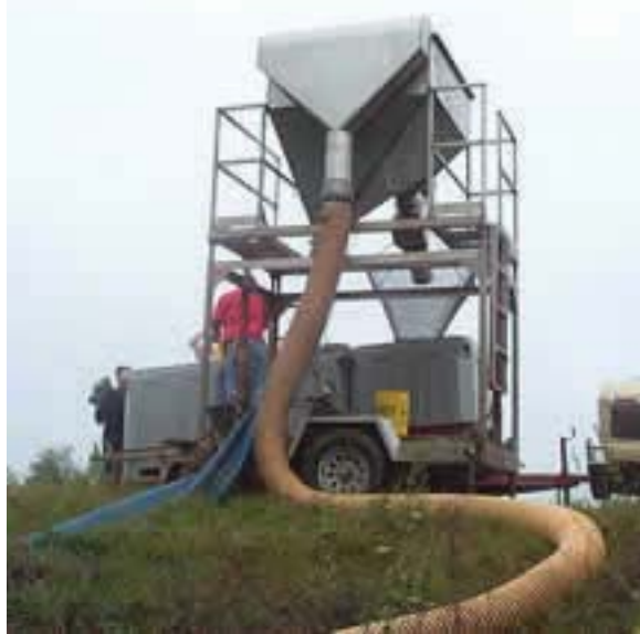
A dewatering tower separates the shrimp from the water at harvest.
